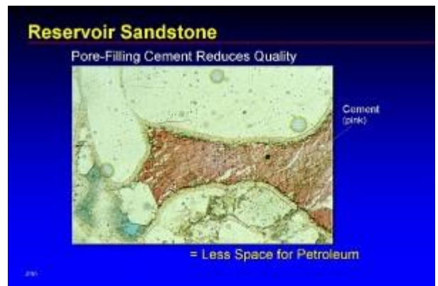
Figure 2: A reservoir rock is one in which pore space exists for the accumulation of hydrocarbon, and the pore spaces are interconnected (permeability) so the hydrocarbon can move both into and out of the pore spaces. Understanding of diagenetic processes and predicting diagenetic histories within three dimensional reservoir facies is essential for optimal reservoir development strategies. © Exxonmobile
